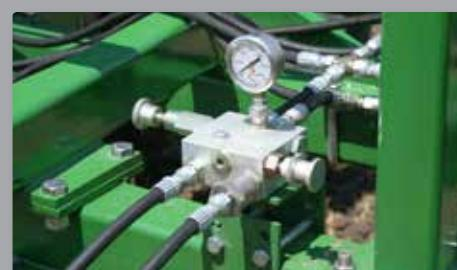
**HYDRAULIC WEIGHT TRANSFER** - Transfer valve adjusts weight from center to wings, providing even, constant down pressure to the full width.
