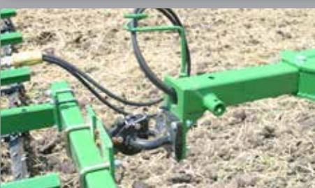
**SINGLE HYDRAULIC CIRCUIT** - This feature allows a simple and quick way to attach to the host machine.
