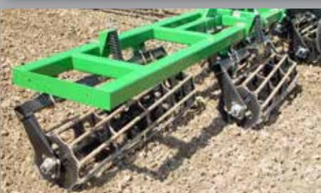
**SPRING-CUSHIONED REELS** - Provide maintenance-free pivot points.
