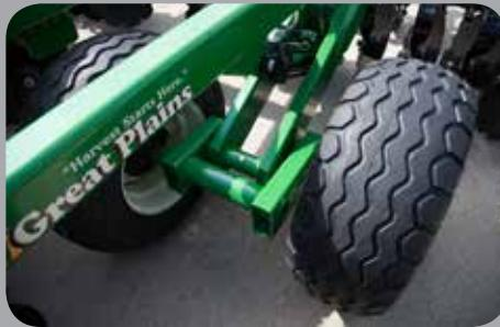
**WALKING TANDEMS** – Provide excellent flotation and safe, reliable road transport.
