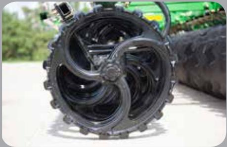
**CONSOLIDATION WHEELS** – Create a fine finish while consolidating the ground just below the surface.
