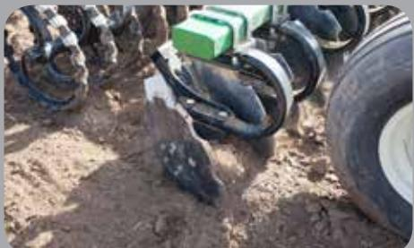
**INDIVIDUAL DISC MOUNTS** – Offer more space between discs for excellent trash flow and better performance in wet conditions.
