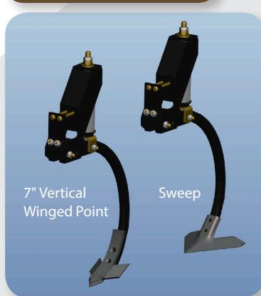
**SHANKS** - Feature 30" of underframe clearance as well as 900 lb trip force to stay in the ground. Points include a 2" Straight Point, a 7" Vertical Winged Point, or 12" or 16" Sweeps.
