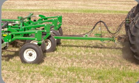
**FLOATING HITCH** - Allows Implement to negotiate undulations independently of the tractor for better ground gauging and depth control.
