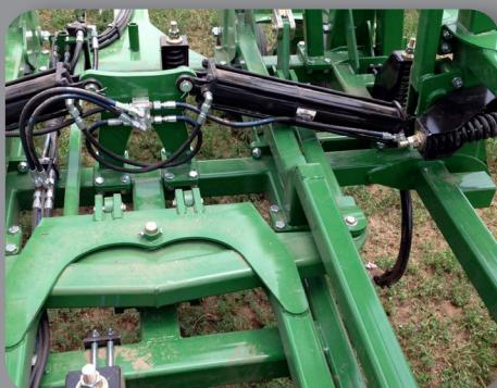
**ROCKING BOLSTER** - Patent-pending rocking bolster-type center frame keeps all center frame wheels on the ground, all the time, regardless of terrain.
