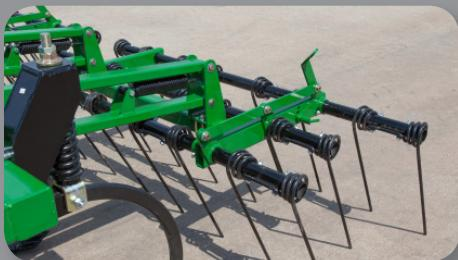
**HEAVY-DUTY SPRING TINE HARROW** - Three-position adjustable heavy-duty spring tines allow the operator choices in tine angle. Longer tines increase trash flow.
