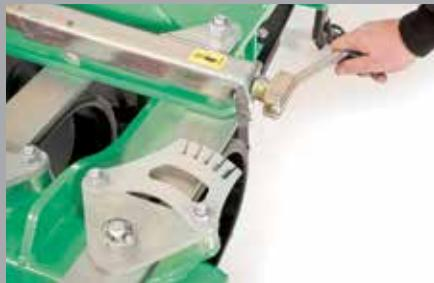
**INFINITE DISC ANGLE ADJUSTMENT** - Disc angling combined with an inclined disc axle allow the X-Press to achieve the same work with a disc that has a smaller diameter and far less concavity. It penetrates the soil and mixes residue while creating less compaction than conventional short discs.
