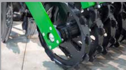
**MAXLIFT ROLLER** - By combining notched wheels and teeth to drive and lift high volumes of soil, the MaxLift Roller creates a fine finish while consolidating the ground just below the surface. This roller achieves a good mixing effect at high speeds.
