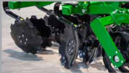
**EXCELLENT TRASH CLEARANCE** - With a massive amount of clearance between both gangs of discs and the rear roller, the X-Press can deal easily with high volumes of trash.
