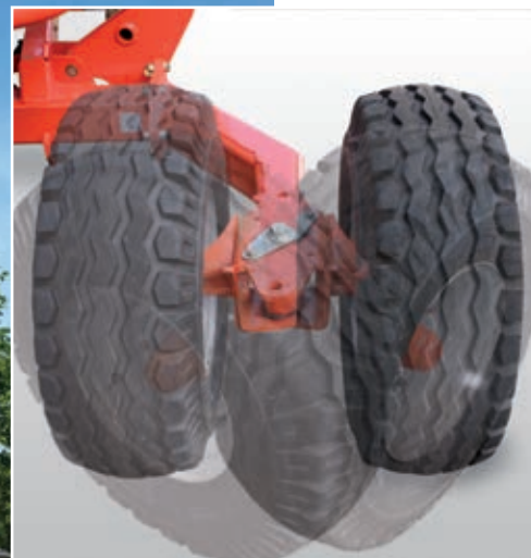
The right-hand wheel can be folded inward for road transport. Left-hand side optional.
