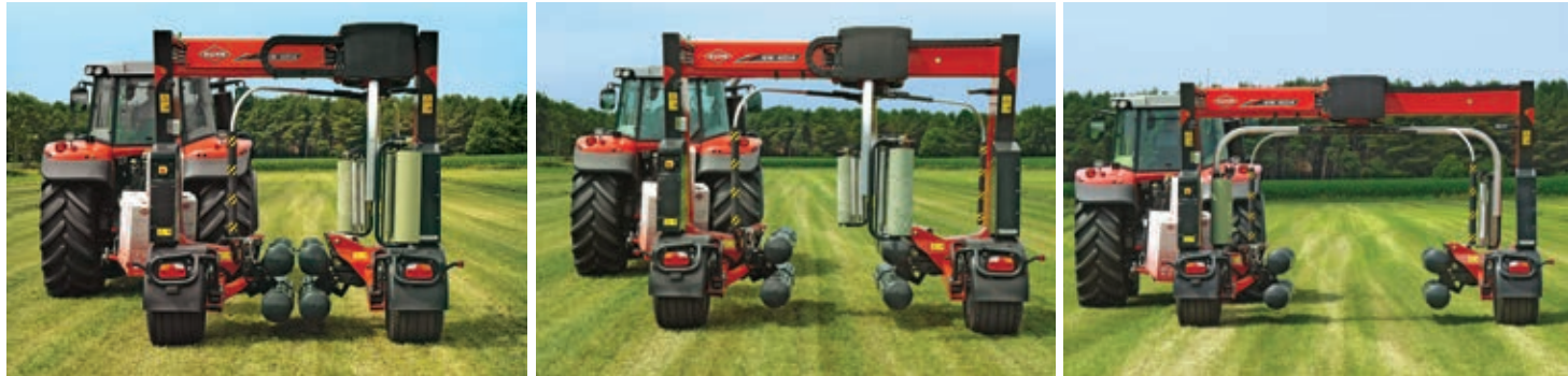
The wrapper folds from its 8' (2.5 m) transport position into 13' (4 m) wide field position.
