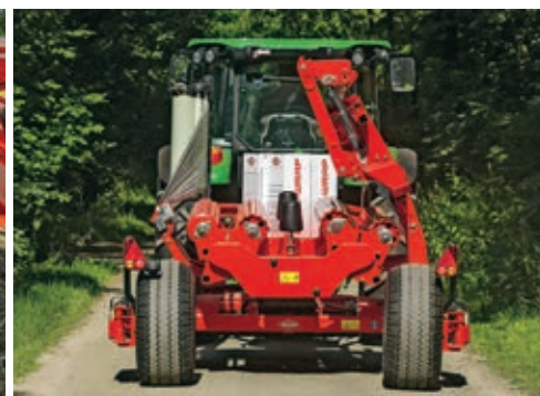
For road transport the wheels can be folded inward to reduce the transport width. Hydraulic folding is optional.
