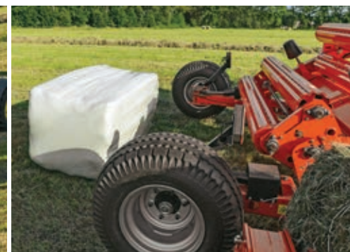
The low table height allows the bale to be gently tipped off to prevent film damage.
