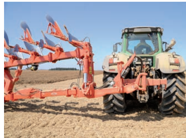
Hydraulic sequencing comes standard meaning fewer valves to operate during headland turns.
