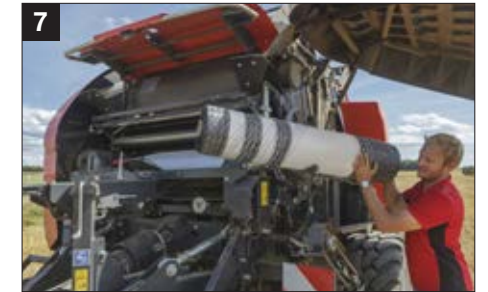
7 Support brackets for easy loading of the net roll
