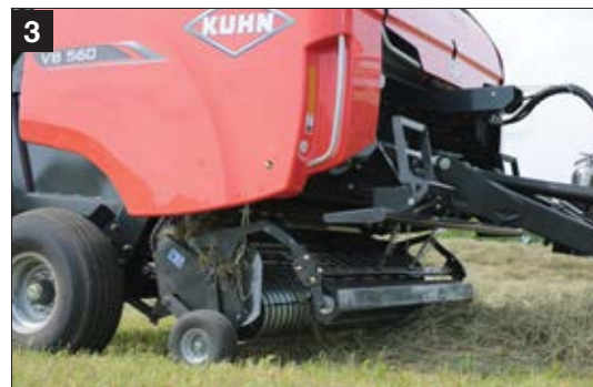
3 90" wide pickup with 5-tine bars to collect all the crop every time
