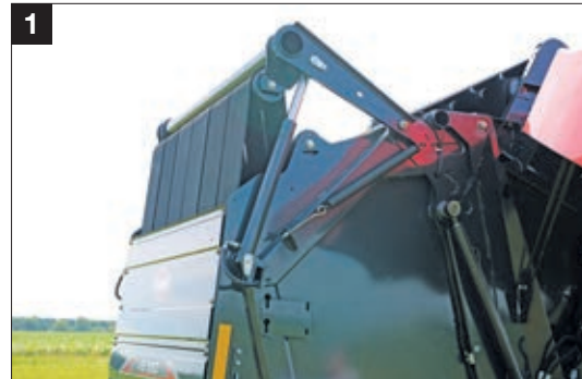
1 Twin tensioning arms provide higher density from improved belt tension control and response time.
