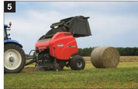
5 Within 4 seconds the bale is ejected and the tailgate is closed again
