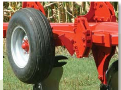
Rear gauge wheel automatically reverses its position as the bottoms rotate.
