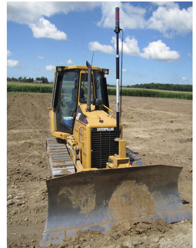
Dozer with EG2-7 mast.
