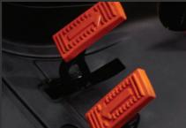
Our hydrostatic drive system (HST) eliminates gear-shifting by safely engaging color-coded forward or reverse pedals. Combining HST with supersmooth joystick control makes front loader work fast and efficient.
