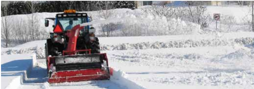
Tivar scraper blade and skid shoes
