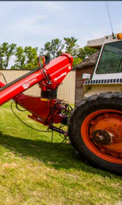
[1] Accessible operating levers [2] Low profile hopper tilts to swing intake into position [3] Posi-Track drive system [4] Hydraulic winch [5] Mounting ring; to fit-up to BackSaver augers [6] Fully retracted [7] Low profile multi-flight hopper
