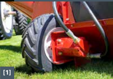
[1] Hydraulic drive wheels [2] Adjustable light [3] Gearbox [4] Auger steer (option)
