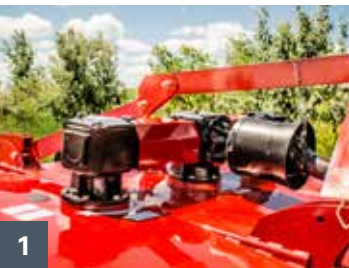
[1] 120 and 90 HP gearbox [2] Standard chain shielding, stump jumper and replaceable front skids [3] 21 inch laminated solid rubber wheels [4] Flat top deck.
