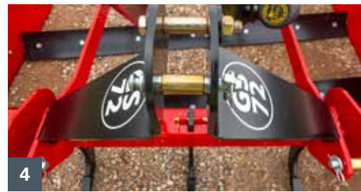
[1] Adjustable scarifier shanks [2] Replaceable and reversible leveling blades [3] Skid shoe adjustments for depth control [4] Heavy duty 3 Pt hitch
