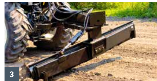
[1] The sideshift feature moves the blade up to 12" off-center. [2] Adjusting the angle on models without hydraulic cylinders does not require tools. [3] The manual tilt adjustment on the 45 Series tilts the blade up to 15°.
