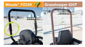
Foldable ROPS (Roll Over Protection System) provides security and protection against roll overs and can be folded down to clear low storage shed doorways vs. Grasshopper's OPS (Operator Protective Structure) which does not fold when necessary to clear obstructions.
