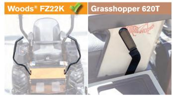
Parking brake integrated into directional control levers engages brake every time handles are moved to outboard position and disengages when moved into operating position vs.
