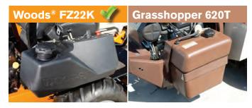
Dual fuel tanks with 8.6 gallon total capacity for longer run time between fill ups and large filler neck on tank makes fill-ups easy vs. Grasshopper's single four-gallon, small opening fuel tank which is harder to fill up and requires filling twice as often.
