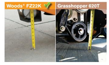
High ground clearance of 7.5" prevents unit from getting hung-up on climbing curbs, or loading onto trailers vs.
