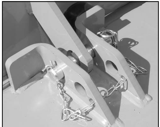
Figure 3. Transport Lock-Up, Left Wing
