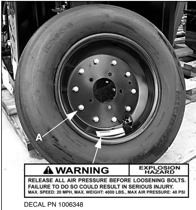
Figure 15. Split Rim Tire Servicing
