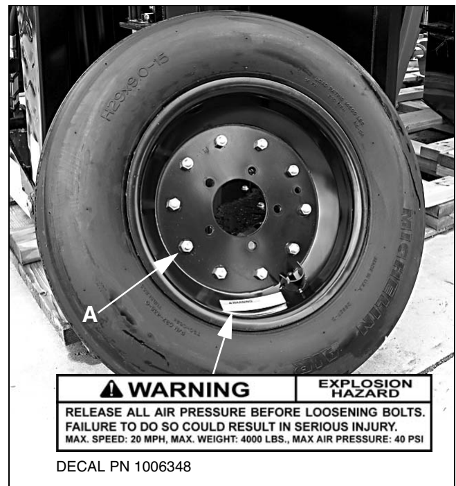
Figure 16. Split Rim Tire Servicing
