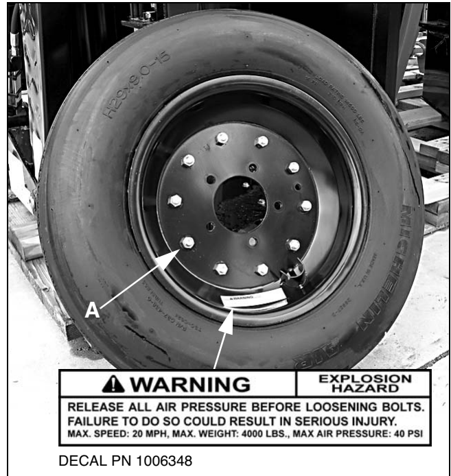
Figure 28. Split Rim Tire Servicing
