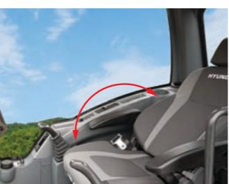
Increased Tilt Angle of Operator's Seat
