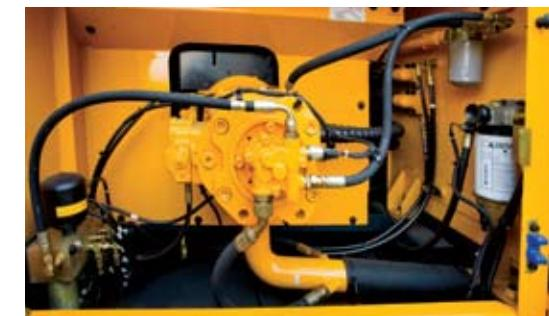
To achieve optimum precision, Hyundai redesigned the hydraulic system to provide the operator with super fine touch and improved controllability. Improved pump flow control reduces flow when controls are not being used to minimize fuel consumption.
