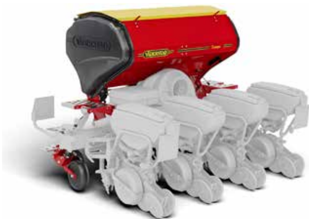
Tempo R can be equipped with a 1200 litre fertiliser hopper and disc fertiliser coulters.
