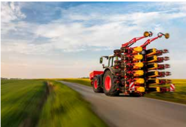
All Tempo V models are vertically folded to 3 metre transport width.
