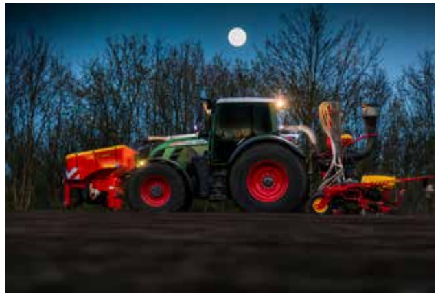
In combination with the front hopper FH 2200, Tempo V is able to combi-drill fertiliser at high speed.
