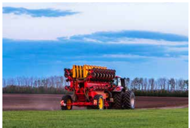
Despite its enormous capacity on the field, Tempo L folds to 3 metre transport width.
