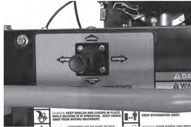
Deflector Control Switches
