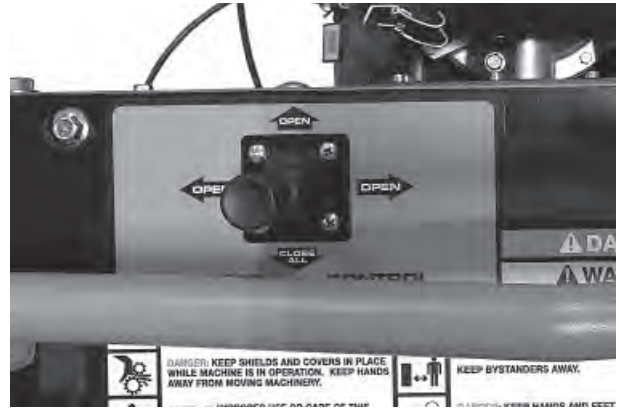
Deflector Control Switches
