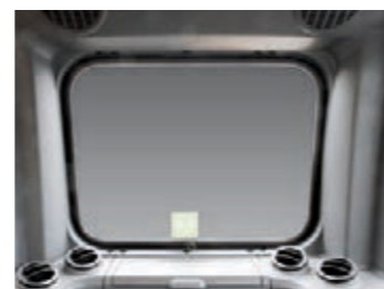
Rear Window Emergency Exit
