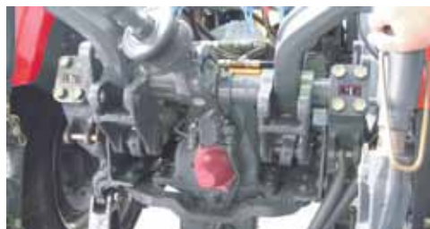
PTO 540-1000 rpm 8 Pin Transmits 96% Engine Power
