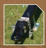
**Standard**5000lb hitch jack, safety chain, slow moving vehicle sign, plated grade 8 fasteners, transport safety locks, gang wrench (2), and separate fore/aft and transport level controls.
