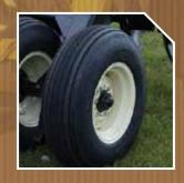
**Hubs/Tires**9.5L x 15 8 ply (load range D X 4) highway implement tires mounted on 6 bolt hub assemblies.
