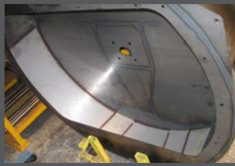
STAINLESS STEEL TURBINE LINER
