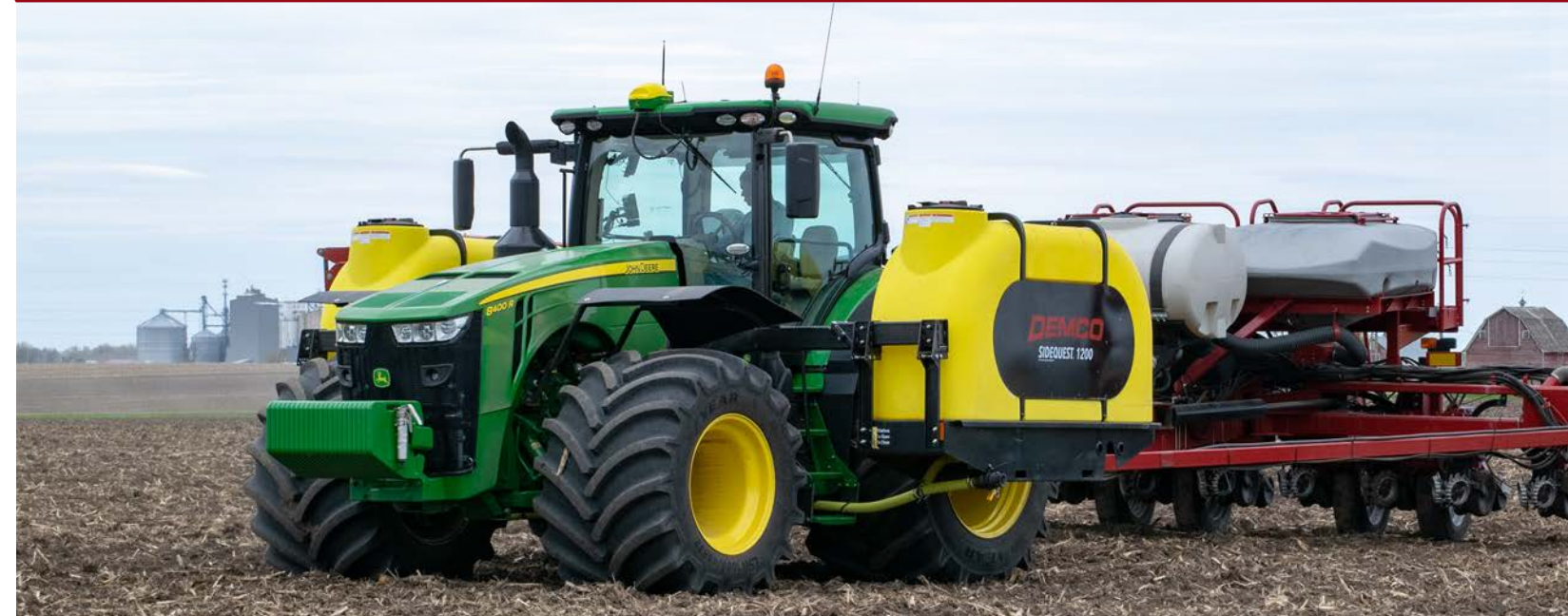
Demco's 300 Gallon Single Axle Sprayer with a 21', 30', or 40' boom has polyethylene elliptical tank with two dual jet agitators and sump.
