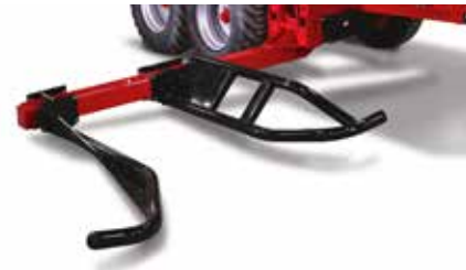
Adjustable tubular loading arm
