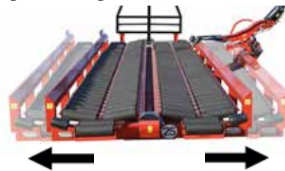
Bale guide adjustable hydraulically
