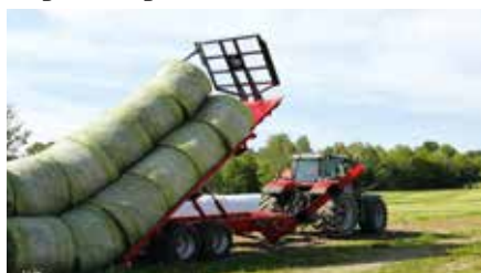
Effortless gravity unloading at 40 degree angle
