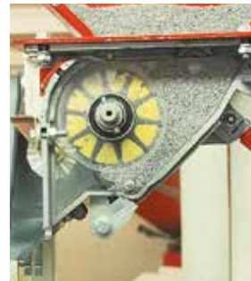
Setting for fine seeds, with rotary brush
