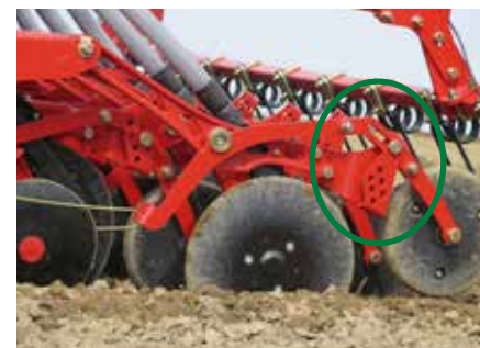
Lifted press wheel setting
