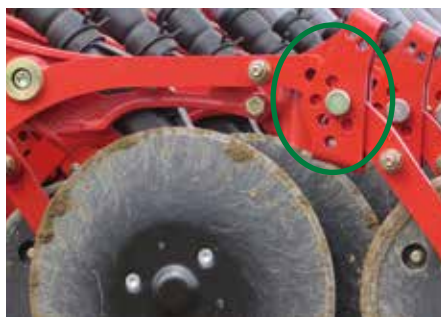
Fixed press wheel setting
