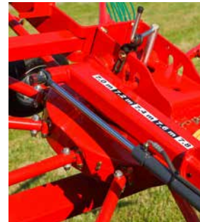
9476 C - Hydraulic 7.0-7.8m working width.
