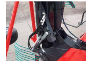
Hydraulic transport locking (optional).
