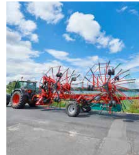
Transport height below 4.0m, even without removing tine arms.
