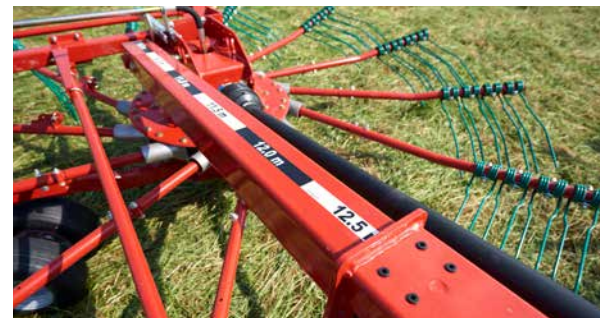
Hydraulic adjustment of working and swath width.
