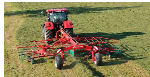
Kverneland 9584 C with 8.40m working width, 9590 C with 9.00m working width, fully enclosed gearbox and hydraulically adjustable working width.
