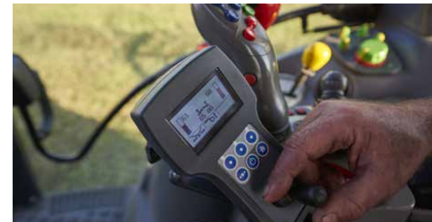
ComfortKit including electronic control of separate rotor height.
