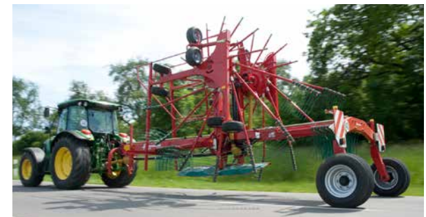
To reach a transport height below 4.00m, the tine arms are removed and safely placed on the carrier frame.
