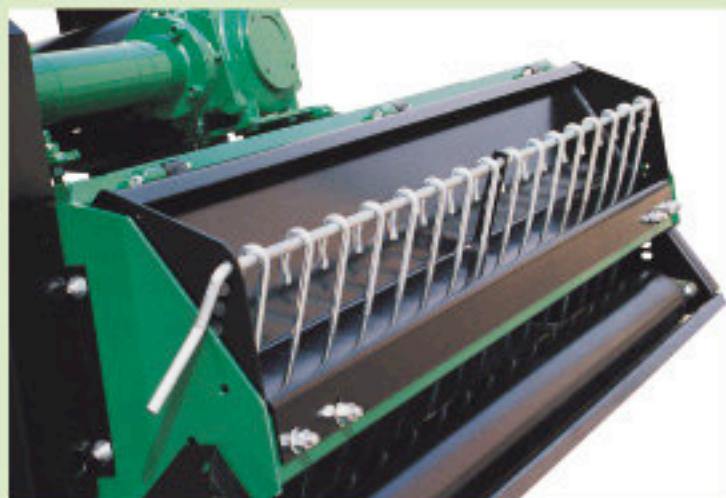
• **Rear shield with spikes.** Choice of knives. Hammers can perfectly crush the branches, thanks to their particular shape and to high rotor speed. Side transmission by special belts. Safety guards.
