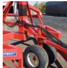
Dolly wheels reduce load on the tongue and improve tracking when pulled behind disc or cultivator.
