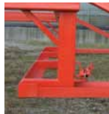
Rear levelling frame is set forward from chassis frame to reduce plugging.
