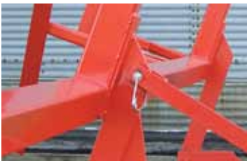
Locking pin simply secures wings in upright position for transport.
