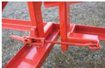
Over-centre clamp locks down the wing into a level, rigid position for levelling.
