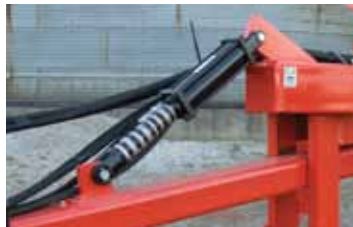
Hydraulic cylinder on tongue adjusts the tongue levelling depth from the tractor.
