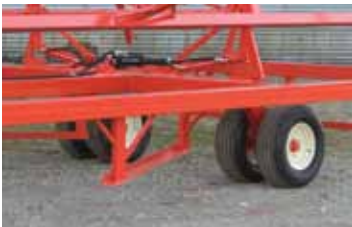
Dual transport wheels provide smoother ride when roading.
