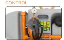
Simple and durable, it keeps the correct pressure in the circuit and ensures the application quality.
