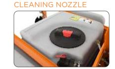
It rinses containers with agrochemical solution under pressure. It incorporates agrochemical residues from containers to the solution in the tank.
