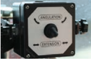
Electrically controlled hydraulic selector valve to adjust raking width and windrow width from the tractor cab
