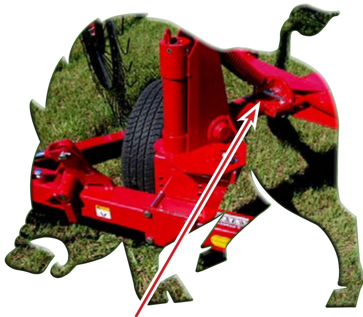
Spring adjustment for finger wheel ground pressure
