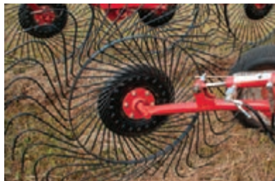
Center wheel kit - hydraulic lift
