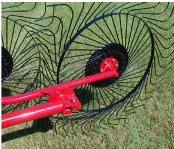
Wheel flotation for uneven ground
