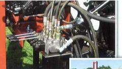
Offset controls allow the operator to stand safely to the side of the unit while posts are being driven.
