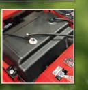
9 gal under the seat fuel tank for improved weight distribution, lower center of gravity, and improved ride
