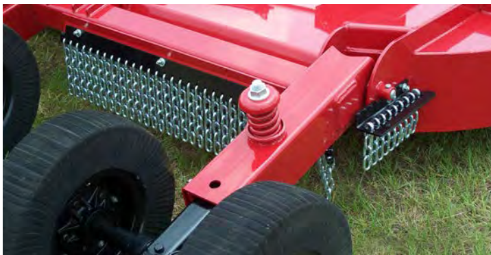
Each axle arm has a strategically placed spring cushion to absorb shock loads near the wheels.
