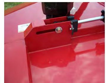
The "free wing float" slot allows the wing to float up and down without moving the hydraulic cylinder rod. This extends the life of the cylinder components.
