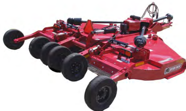
Each axle arm on the center section has a rubber cushion to absorb the shock loads near the wheels. Shown with optional dual tires on the center.
