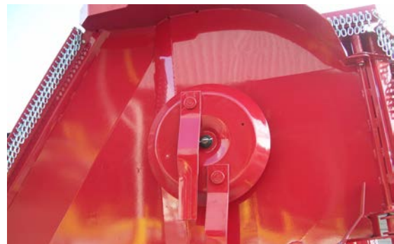
The design of the wings adds exceptional strength in the gearbox stands without the use of exposed structure.
