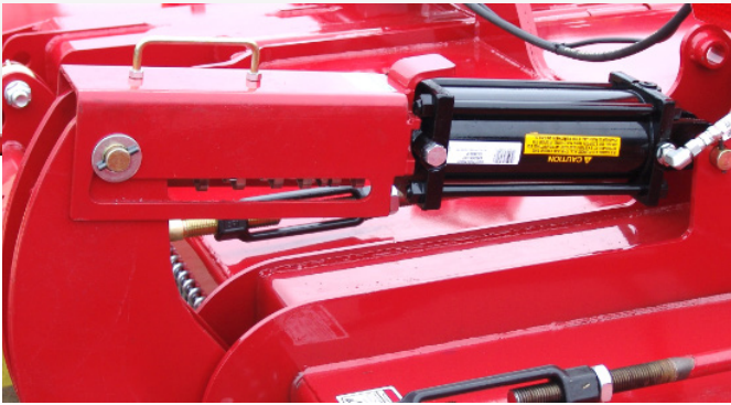
The transport lock-up device is easily positioned to take the load off the hydraulic cylinder rod during transport.
