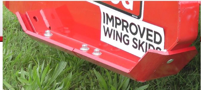
The wing skids are in two pieces for more economical replacement and the 45 degrees of up- turn allows the skid to float over the ground instead of gouging in. This prevents possible damage to the sideband.
