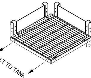
**STEP 1: BOLT THE PLATFORM TO THE TANK**
