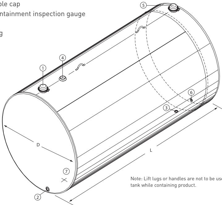
Note: Lift lugs or handles are not to be used to move tank while containing product.
