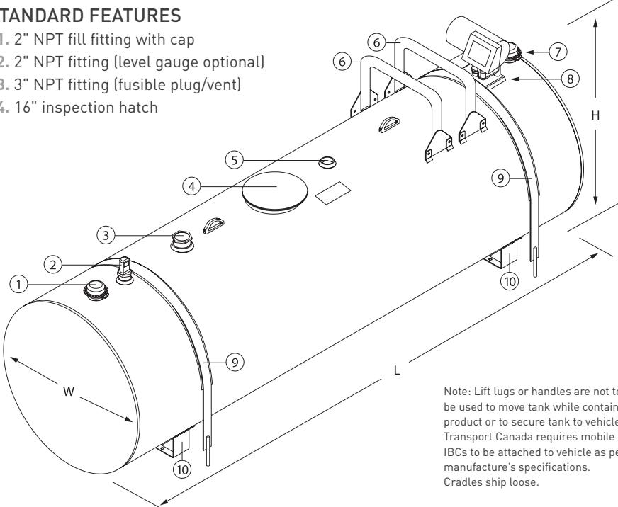
Note: Lift lugs or handles are not to be used to move tank while containing product or to secure tank to vehicle. Transport Canada requires mobile IBCs to be attached to vehicle as per manufacturer's specifications. Cradles ship loose.
