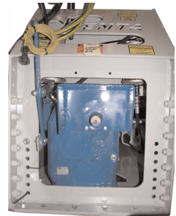
SD Tornado Auger Auger Thickness 1/2" (Option 3/4")
