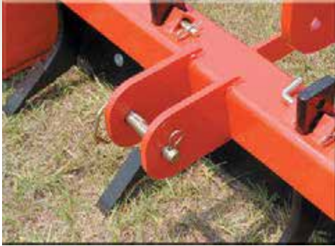
Scarifiers can rip soil up to 2-3/8" deep.
