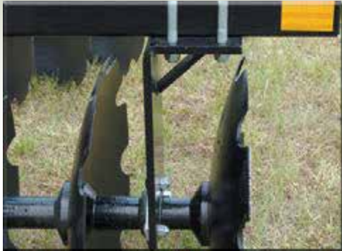
Bearing hangers reinforced with gussets
