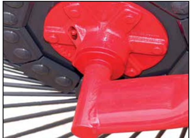
An anti-wrap seal protector on the backside of each finger wheel hub adds more protection for the seal and bearing.
