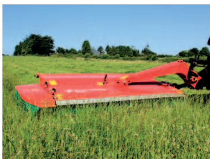
Centre suspension for even weight distribution across the entire working width.
