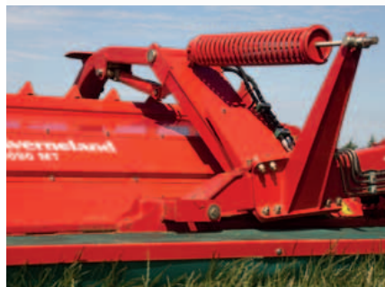
The Kverneland NonStop BX-Belt system, with individual BreakBack of each rear mower.
