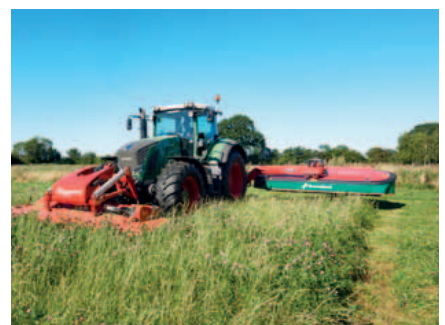
Adjust lifting height on headlands. In low crop conditions the lifting height of mowing units can be reduced for even faster headland operations.
