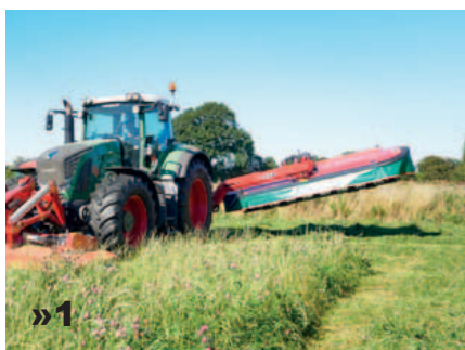
»1 Minimum 500mm ground clearance across the complete mowing unit during headland turns. Mowing unit is raised and carrying arm tilted to a 10° angle.
