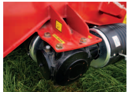
540/1000rpm turnable gearbox as standard.
