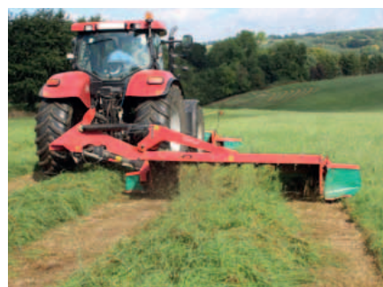
The large compensating spring ensures excellent flotation across the full mower width.
