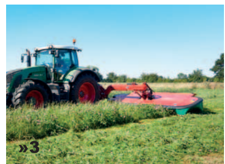
»3 Mowing unit is lowered evenly onto the ground without one side touching the ground before the rest of the mower.
