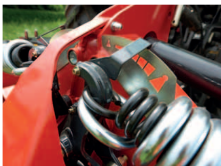
Large suspension springs, optionally with hydraulic setting of ground pressure.
