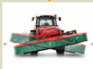
Vertical adaptation of 24° to adjust to uneven fields.
