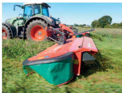
New FlexProtect sidecovers, rugged and sturdy, yet flexible if bumping into obstacles.
