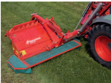
The centre suspension of the two rear mowing units provides excellent ground following.
