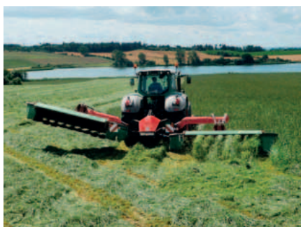
Each mowing unit can be lifted individually, convenient when mowing awkward shaped fields.
