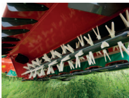
Efficient nylon tine conditioning.
