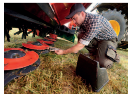
Easy and quick access to the cutterbar for daily inspection of discs and knives.
