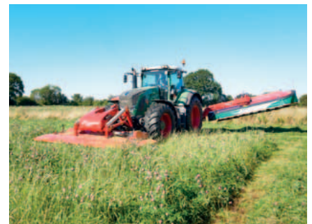
Automatic headland control – front mower is lowered before the rear mowing units.
