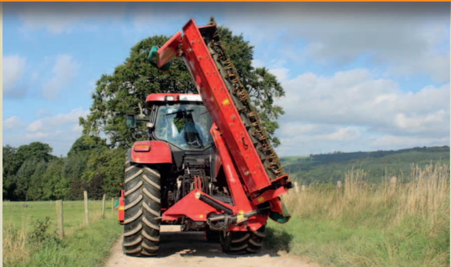
Kverneland 3200 series is folded into a vertical transport position using a hydraulic cylinder.
