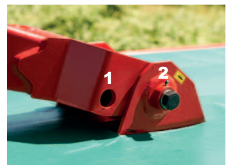
Two mounting positions of cutterbar on suspension for optimal overlap.
