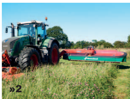
»2 The carrying arm is tilted back to bring the mowing unit into an even position before lowering the mowing unit.
