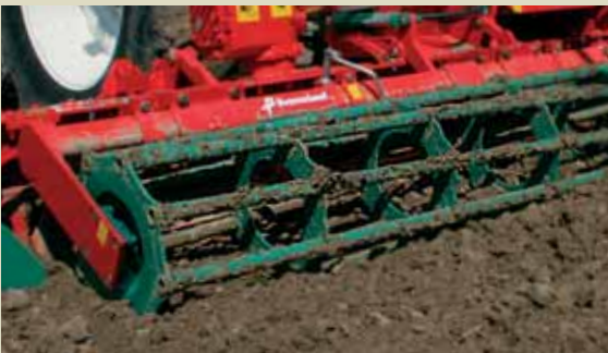
Cage Roller Ø 550mm
