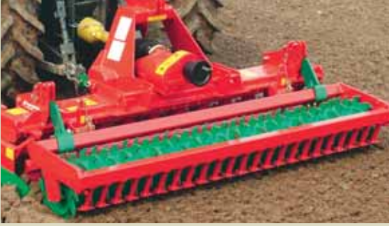
Tooth Packer Roller Ø 500 + 585mm
