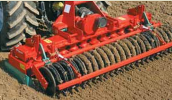
Cracker Roller Ø 550mm
