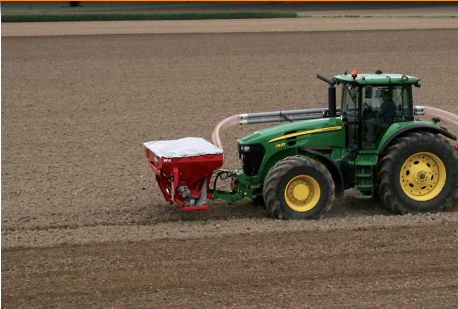
Kverneland NG-S F35 and Kverneland Accord DF-2 coulter bar with front hopper
