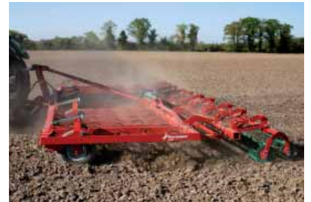
The double crumblor rollers are mounted on a parallelogram. The rollers have two different diameters, larger at the front - smaller at the rear, for improved clod breaking.
