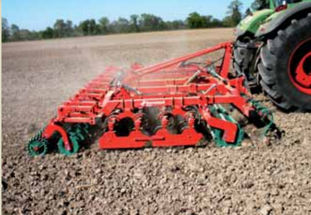
TLG equipped with Clod Board and combination of crumble and crosskill roller.
