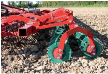
The double crumblor rollers are mounted on a parallelogram. The rollers have two different diameters, larger at the front - smaller at the rear, for improved clod breaking.
