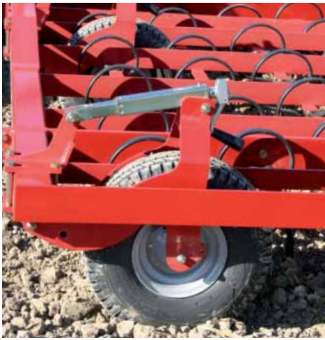
The working depth can be easily and precisely adjusted by crank.
