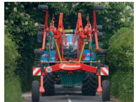
The centre swath rakes are converted hydraulically for transport position from the tractor cab. Tine arms are removable.
