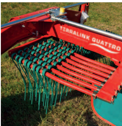
Kverneland Taarup 9476 C - Easy storage of tine arms for transport.
