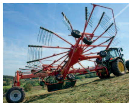
The two rotors are hydraulically lifted on headlands, and ensure outstanding ground clearance in headland position.
