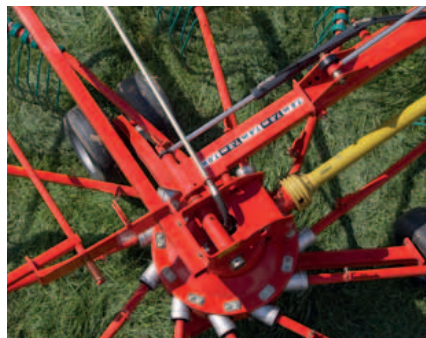
The working width is hydraulically adjustable from the tractor cab on all models.
