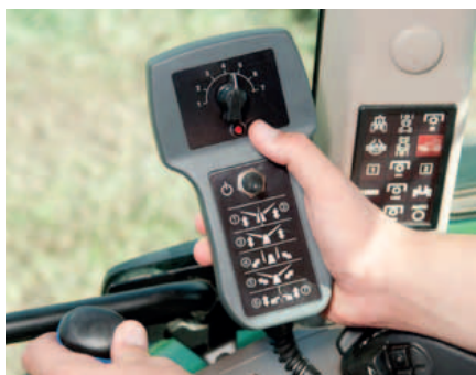
The control box, placed in the tractor cab, controls the main functions needed during work. Lift and height adjustment of rotors can be done individually. Working width can be easily adjusted, and the box also features a transport locking device.
