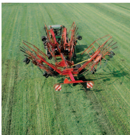
Conversion from transport to working position is very fast, and is carried out from the tractor cab.
