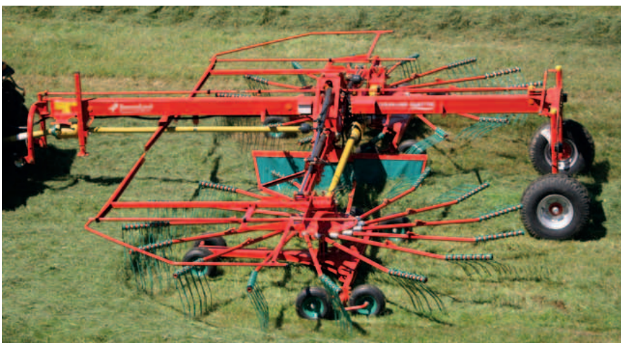
The Kverneland Taarup 95110 C is fitted with the TerraLink Quattro system, offering perfect ground contour followings. A unique combination of an undercarriage with 6 wheels and a specially designed rotor suspension, ensures superb raking
