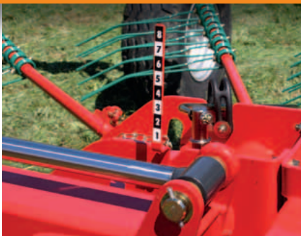
Hydraulic height adjustment of the rotors to suit length of the stubble or varying ground conditions.
