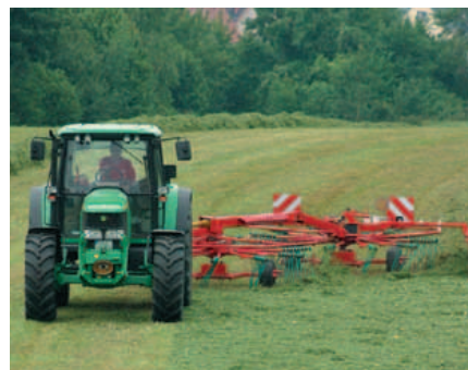
SideShift to the left - raking without driving on unraked crop.
