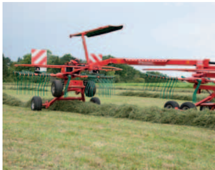
Turning on headlands: Kverneland Taarup is equipped with the QuickLift system as standard. This ensures a lifting height of 50 cm to easily over cross existing swaths.
