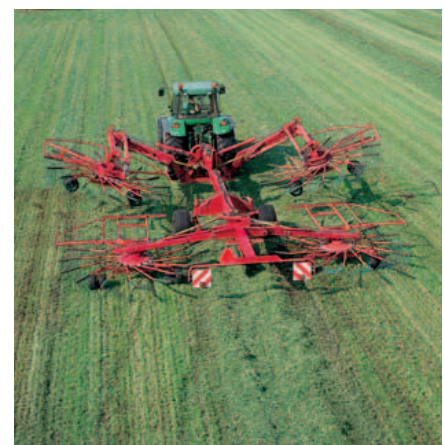
The rotors can be lifted sidewisely (inner and outer rotor at the same time). Crossing swaths without damaging them is no problem with the 15 m rake.
