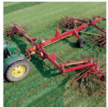
The two outer rotors can be adjusted individually.
