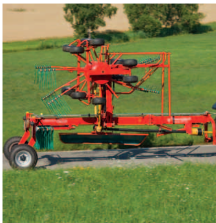
The centre swath rakes are converted hydraulically for transport from the tractor cab. To limit transport height further, the tine arms can be detached on the 9476 C. The swath board folds up automatically.
