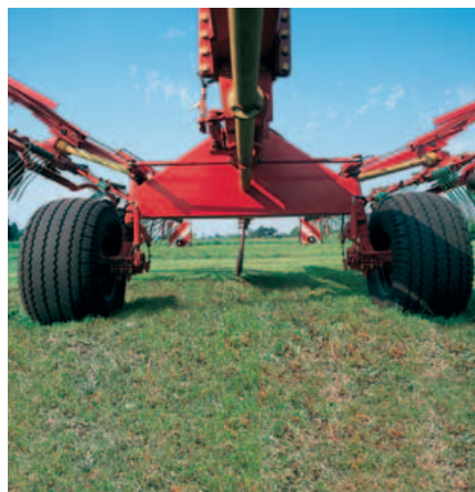
The giant balloon wheels (up to 550/45R-22.5) of Kverneland Taarup 95150 C come optionally with active steering wheel axles for outstanding manoeuvrability.
