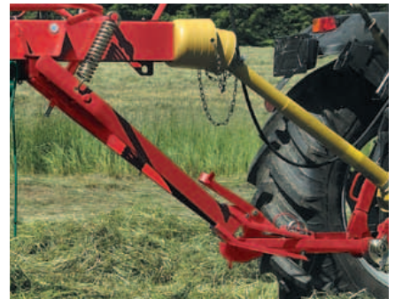
Both rakes are equipped with a double, wide angle PTO shaft – for increased manoeuvrability.
