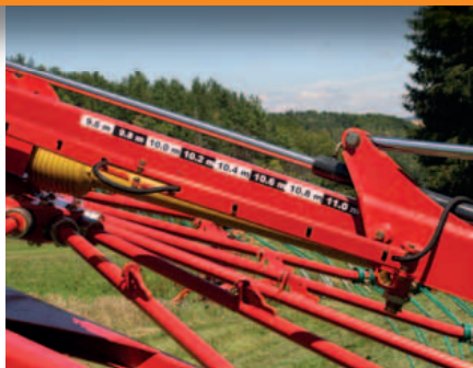
Hydraulic adjustment of working width between 9.6 and 11m.
