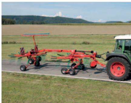
Pulled axle suspension for smooth running characteristics and reduced power requirement.
