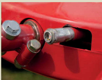
Clearly visible oil level via inspection glass.
