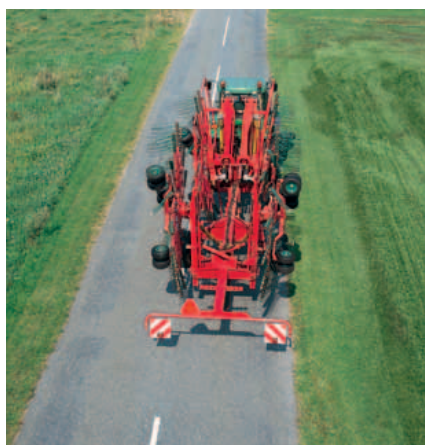
During transport the height of the machines is below 4 m, without removing the tines. Transport width with detached tine arms is only 3.45 m.
