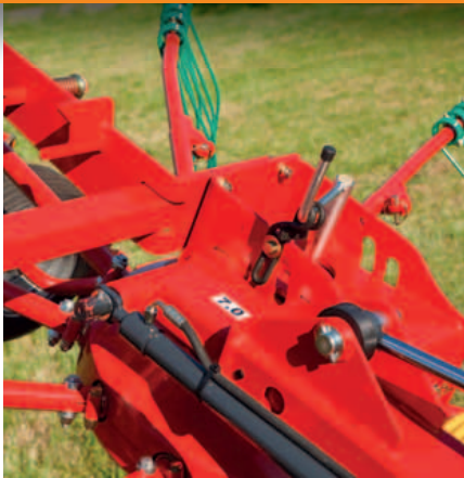
The hydraulic adjustable working width can be set between 7.0 m...
