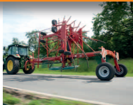
To reach a transport height below 4 m, the tine arms are removed and safely placed on the carrier frame.
