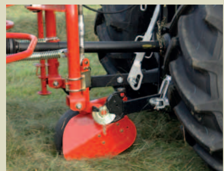
As an option these rakes can be supplied with a third wheel, which can be easily adjusted from the top and allows continuous use of the standard top link.
