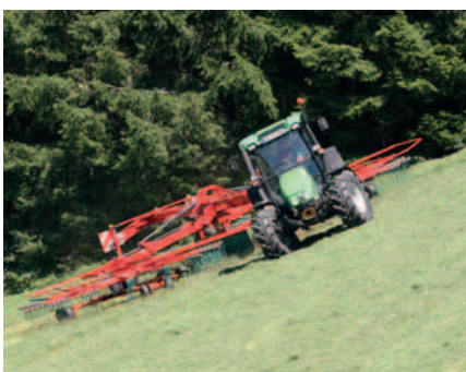
Active wheel steering, allowing sharp turns on headlands and during transport.
