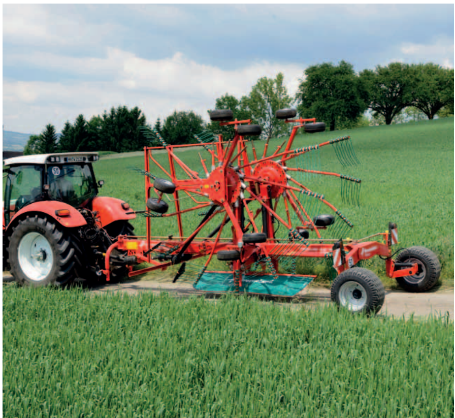
Due to the Hydro axle Kverneland Taarup 9590 Hydro has a transport height of less than 4.0m, even without detaching the tine arms.
