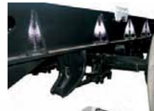
HD Spring Suspension (Hiway Commercial)
