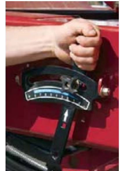
Air valve control at each meter enhances accurate delivery of products that may vary in size and weight. In-cab control is an available option.
