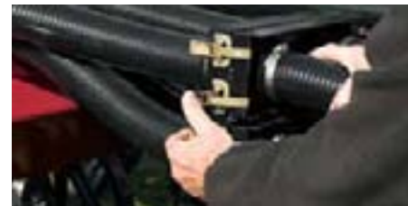
Quick-connects let you hook up to seeding or banding tools quickly and easily.
